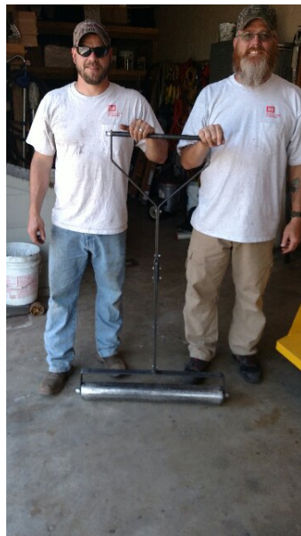
Hannibal maintenance mechanics display the built-from-scratch roller for installing the new roof membrane
